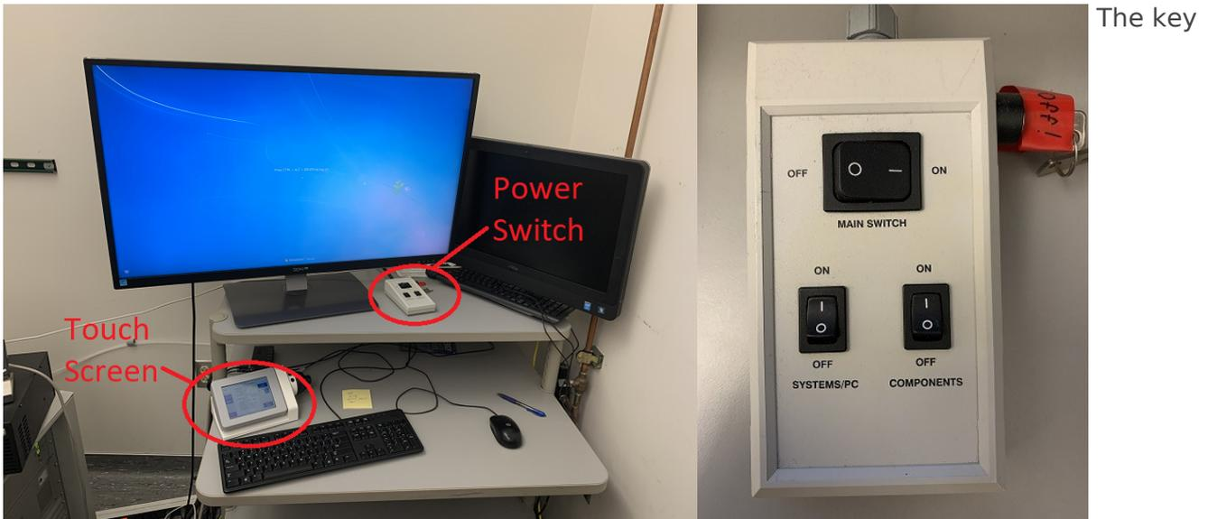
Turn on the X-Cite lamp next to the microscope. Turn on the Argon ion laser. Turn the key to the horizontal position and flip the small metal switch up. If the light is red lower the current control knob until it is green.
