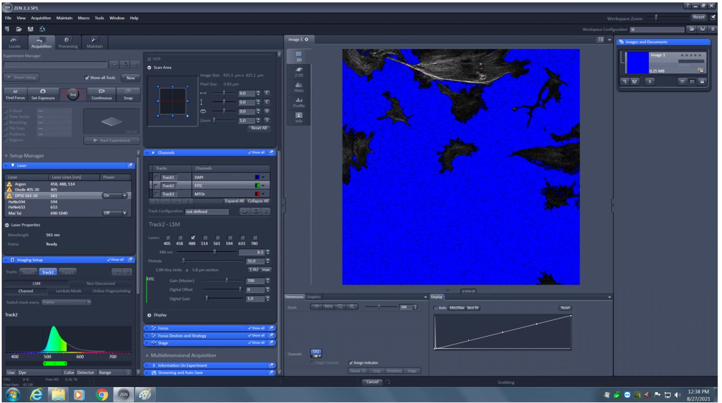
Press the "stop" button, and repeat this procedure for the other channels. Once you are done setting up all the channels we will setup the scan parameters in the acquisition menu
