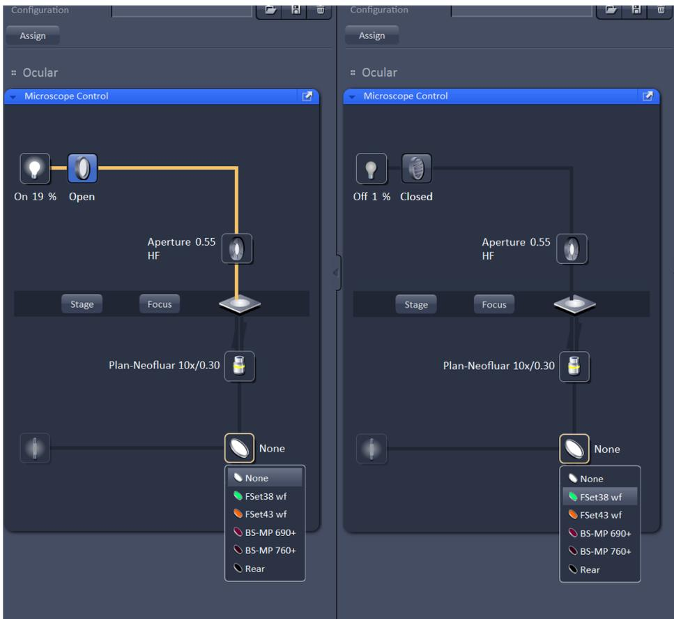
You can also use the touch screen to control these settings and view the sample in the eyepiece. The main menu on the touch screen will display information about the objective and stage position. There is also a button labeled "Make It Visible" that will put the microscope directly into a bright field configuration so you can view the sample.
