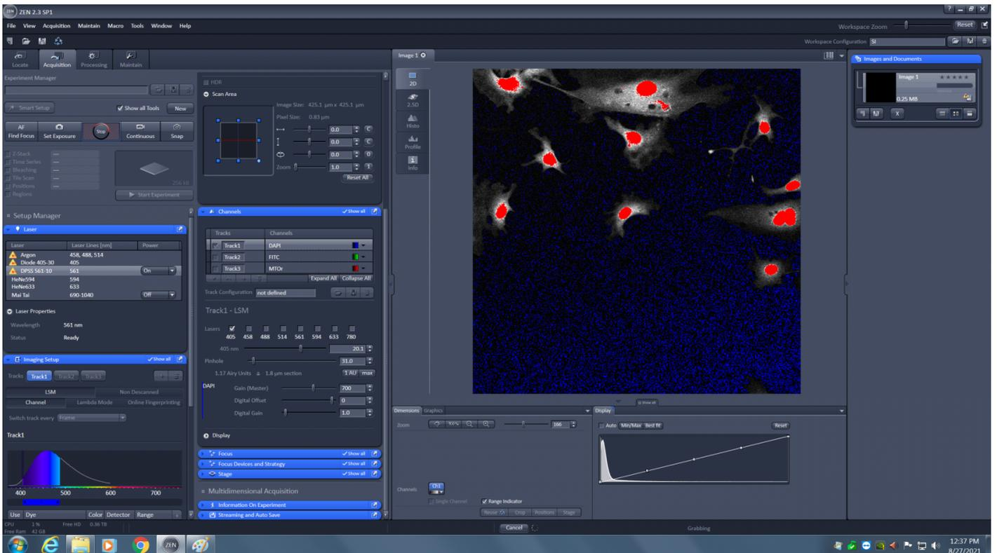
Maximize the amount of red to make sure your sample is in focus. Then lower the laser power to that only a few red pixels are visible. You want to use as much of the detector's dynamic range as possible without saturating the detector. A few red pixels are okay, you just don't want big patches of them. The correctly adjusted image should look as shown below.
