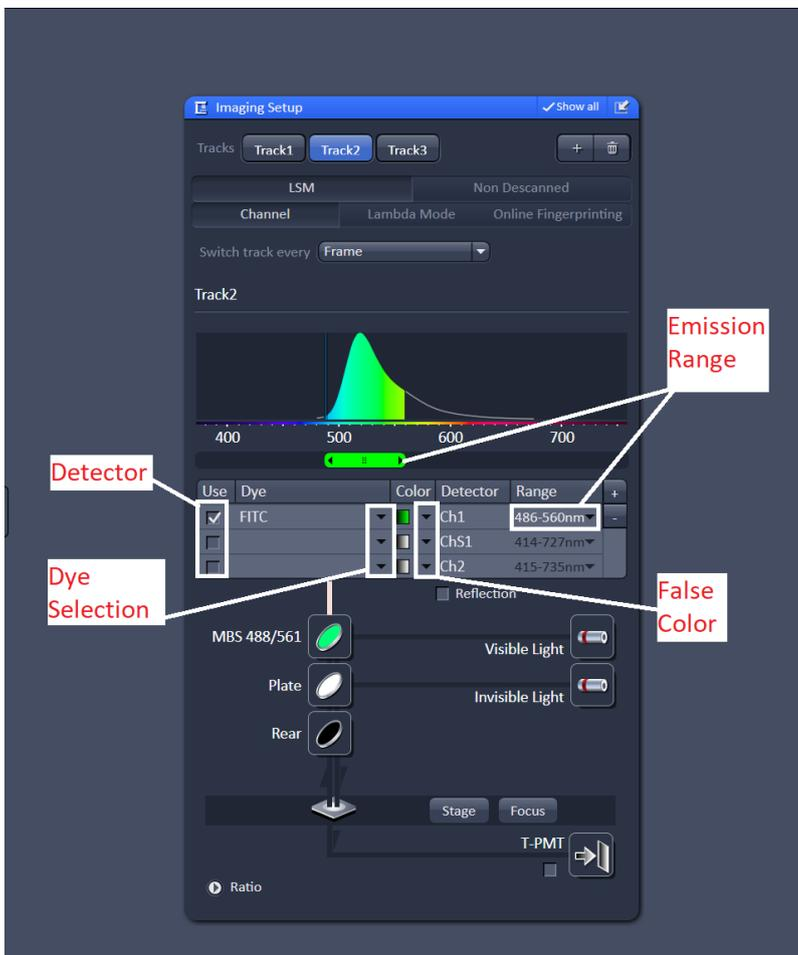
Next, select the detector you want to use. By default channel 1 is selected as the detector. As long as "switch track every frame" is selected you can just leave the detector as channel 1. Choose a dye from the database, this will display the emission spectrum of the dye. Adjust the emission range so that you are collecting most of the light from the emission spectrum. Repeat this for every track - one track for every dye in the sample.
