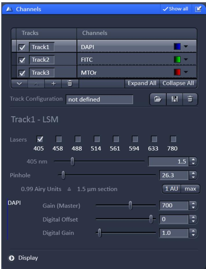
For each channel you will need to adjust the laser power, gain, and pinhole size. Start by setting the gain to 700. Raising the gain will increase your signal but will also increase your noise. Lowering the gain will lower the signal and noise, requiring you to use a higher laser power. We have found that 700 gain is a good starting point.
