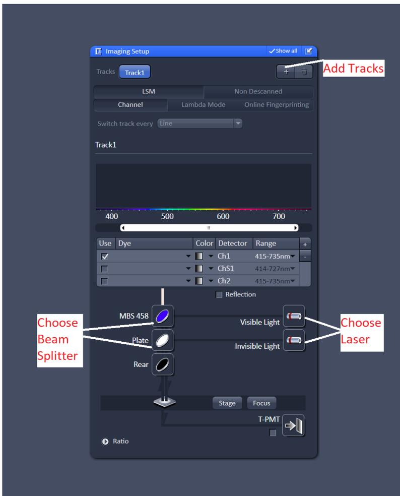
For each track choose a laser. Then choose a beam splitter (dichroic filter) that matches the laser line. For example, if you are using the 488nm laser, choose one of the beam splitters labeled for 488nm.
