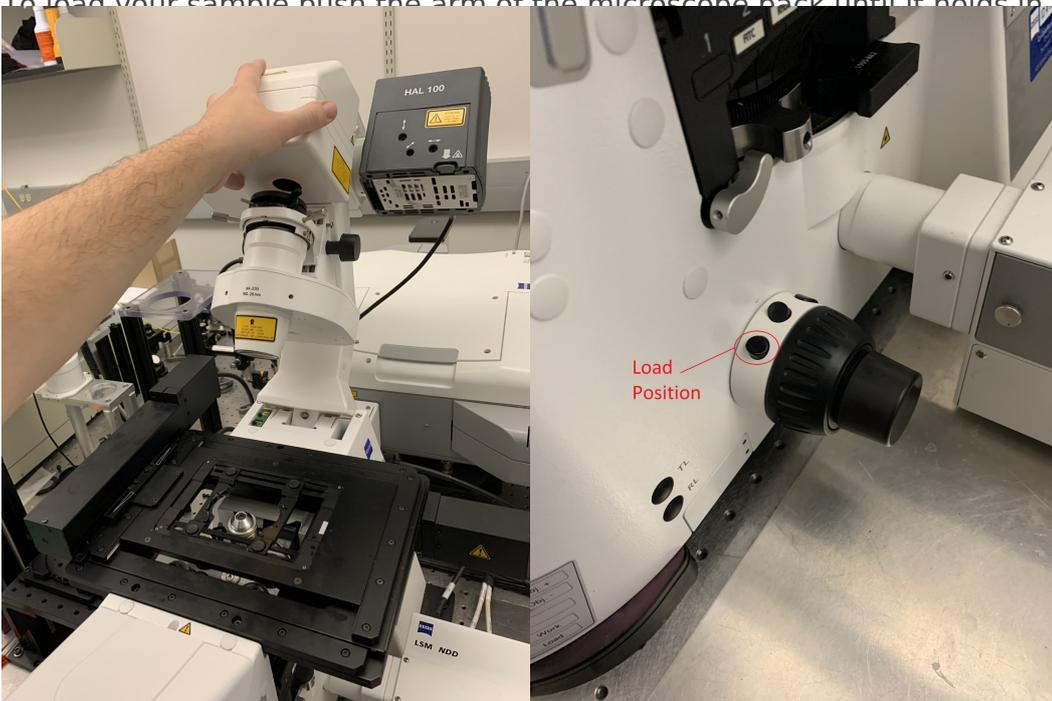
Move the sample to holder to the correct position for either a slide or a 35mm dish. Make sure to load the sample with the coverslip facing down (towards the objective). If you need to use the 40x or 63x objective add a drop of water or immersion oil to the objective lens. After placing the sample on the holder, press the upper button on the focus knob to return the objective to the working position. Lower the microscope arm (there is an interlock that will prevent the laser from turning
